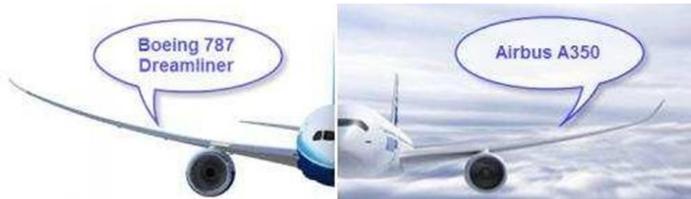
Figure 1.10- Raked wingtips on the new Boeing 787 and Airbus A350.
