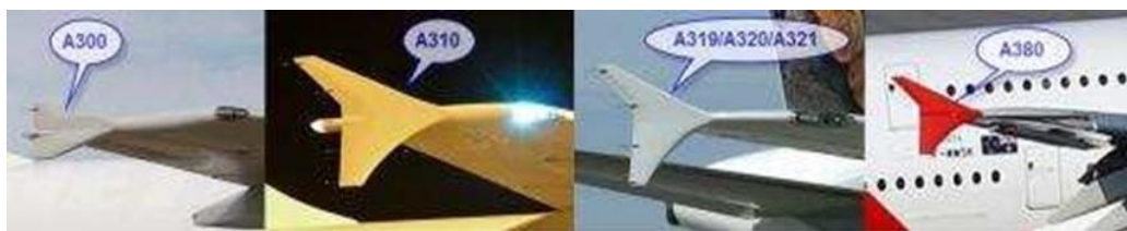
Figure 1.8- Airbus fence Winglets.
