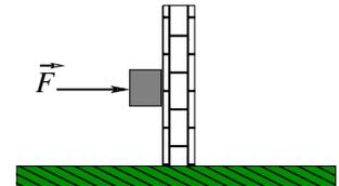
SOLUTION :a) The wall exerts on the brick the static friction force  $\vec{F}_s$  and the normal force  $\vec{N}$ .
