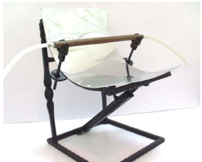
Fig. 5. Photograph of the portable solar collector.
