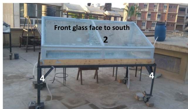
Fig. 1. Front view of the solar still.
