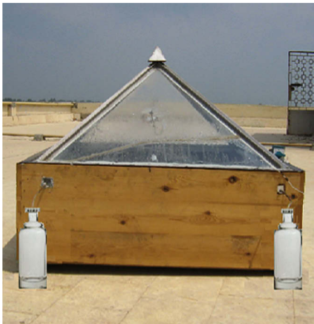
Fig. 2. A photograph of the fabricated concave wick solar still.
