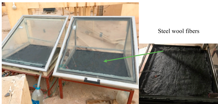
Fig. 3. A photographic of the setup of the solar still with PCM and steel wool fibers.
