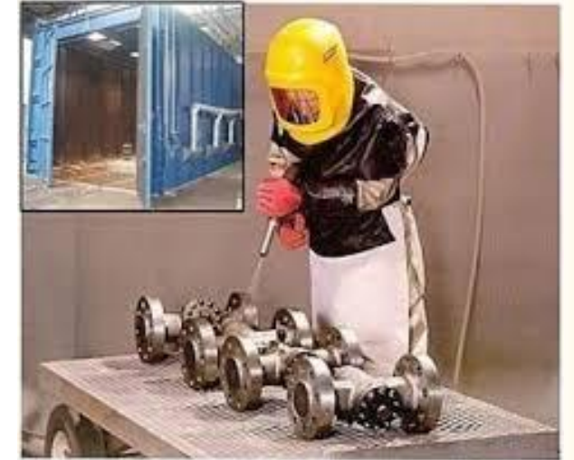
Cabine de grenailage
