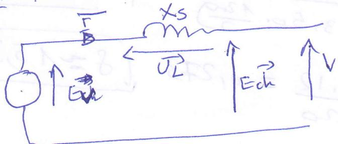
$$\text{Comme } R_s \approx 0 \Rightarrow E_{\text{ch}} = V \Rightarrow |E_{\text{ch}}| = 220 \text{ V}$$
