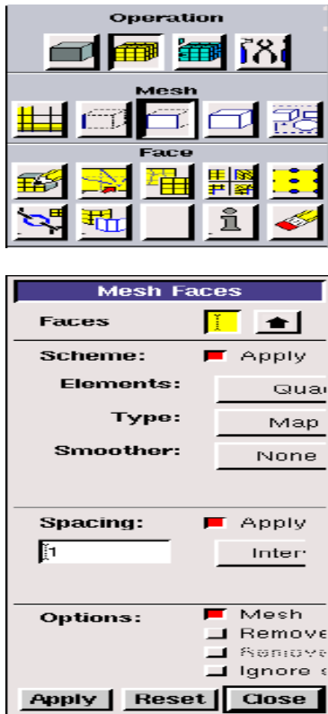
Figure II.4 : Le maillage des faces (GAMBIT Command Reference Guide, 2000).
