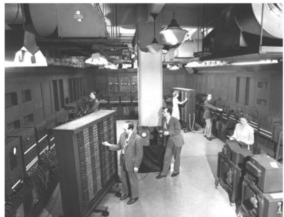
Fig. 7. L'ENIAC - the Electronic Numerical Integrator and Computer (ENIAC) -1943-1946.
