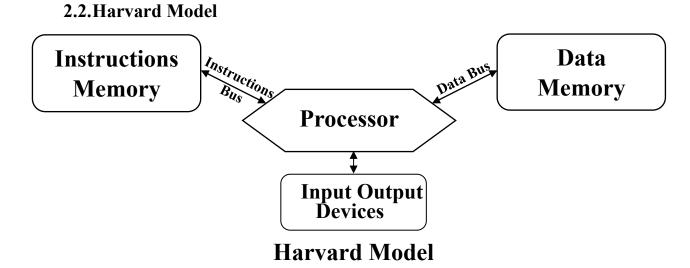
This structure differs from the Von Neumann architecture only in that program (instruction) and data memories are separated. Access to each of the two memories is done through a distinct path. This organization allows for the simultaneous transfer of an instruction and data, which improves performance.
