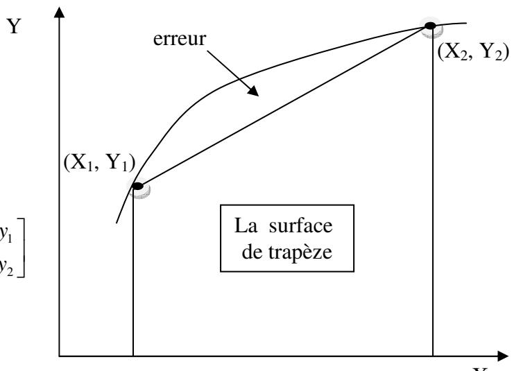
$$\text{La surface de trapèze} = \int_{X1}^{X2} f(x).dx = \int_{X1}^{X2} (C_1 + C_2 \cdot x).dx = \left( C_1 \cdot x + C_2 \cdot \frac{x^2}{2} \right)_{X1}^{X2} = \frac{X_2 - X_1}{2} \cdot (Y_1 + Y_2) = \frac{H}{2} \cdot (Y_1 + Y_2)$$
