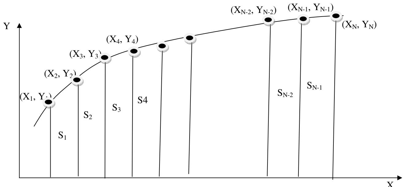
$$\text{La surface Total} = Trap = \sum_{K=1}^{N-1} S_K = S_1 + S_2 + S_3 + \dots + S_{N-2} + S_{N-1}$$
