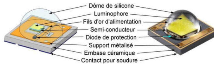
Figure VI.3: Packaging de la LED [38].
