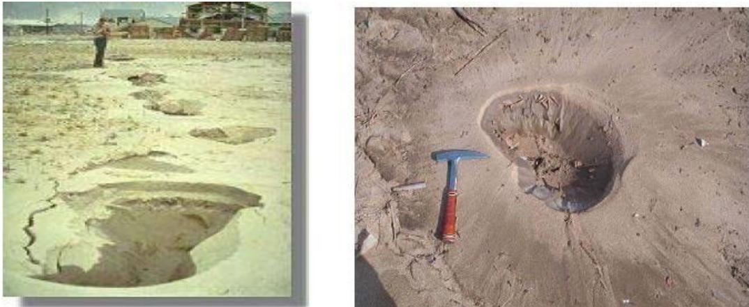
Figure 3.5 Ebullition de sable
