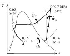
$$\dot{Q}_L = \dot{m}(h_1 - h_4) = (0.12 \text{ kg/s})(246.36 - 84.98) \text{ kJ/kg} = 19.4 \text{ kW}$$
