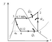
$$\dot{Q}_L = \dot{m}(h_1 - h_4) = (0.05 \text{ kg/s})(236.97 - 88.82) \text{ kJ/kg} = 7.41 \text{ kW}$$
