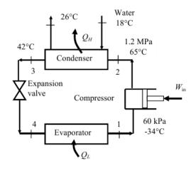
(b) The mass flow rate of the refrigerant may be determined from an energy balance on the compressor
