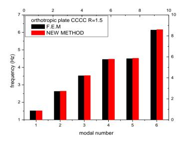
Figure 2: Comparative results of F.E.M and New Method for CCCC orthotropic plate NOTE: This analysis can be extended to all higher modes
