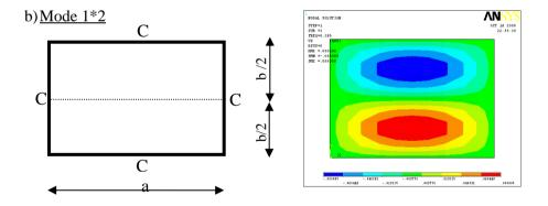
The plate develops a modal sequence with two sub plates CCSC and SCCC where the nodal line position is symmetrical because of the symmetry of the extreme supports CC. The circular frequency for mode 1\*2 is obtained by the following equation:
