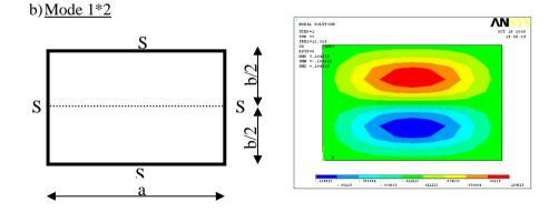
The plate develops a modal sequence with two sub plates SSSS where the nodal line position is symmetrical because of the symmetry of the extreme supports SS.
