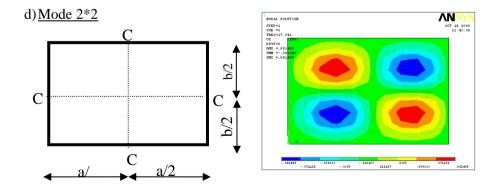
The plate develops a modal sequence with four sub plates CCSS where the nodal lines positions are symmetrical because of the symmetry of the extreme supports CC and CC. The circular frequency for mode 2\*2 is obtained by the following equation:
