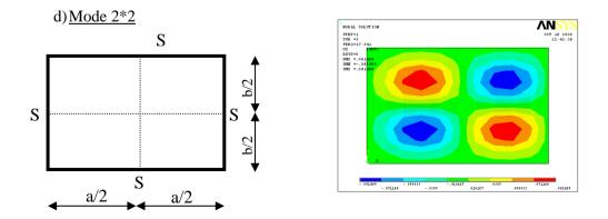
The plate develops a modal sequence with four sub plates SSSS where the nodal lines positions are symmetrical because of the symmetry of the extreme supports SS and SS. The circular frequency for mode 2\*2 is obtained by the following equation:
