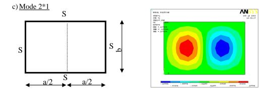
The plate develops a modal sequence with two sub plates SSSS where the nodal line position is symmetrical because of the symmetry of the extreme supports SS.
