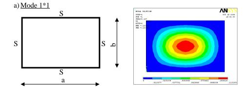
The circular frequency for mode 1\*1 is obtained by the following equation:
