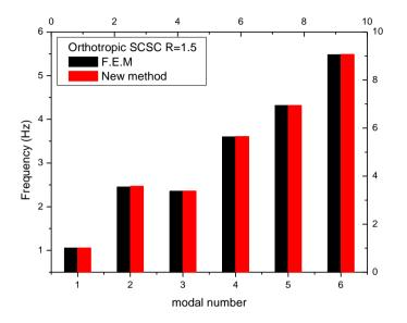
Figure 3: Comparative results of F.E.M and New Method for SSCC orthotropic plate
