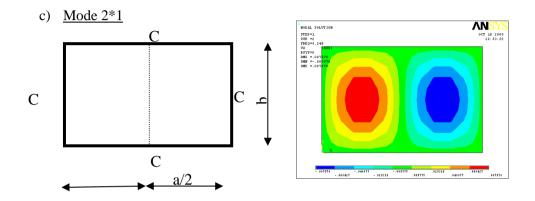
The plate develops a modal sequence with two sub plates CCCS and CSCC where the nodal line position is symmetrical because of the symmetry of the extreme supports EE. The circular frequency for mode 2\*1 is obtained by the following equation:
