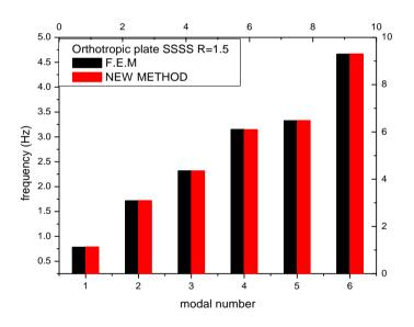
Figure 1: Comparative results of F.E.M and New Method for SSSS orthotropic plate
