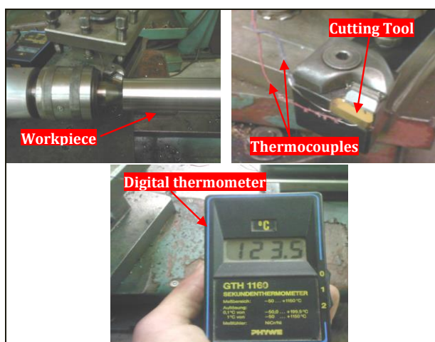
Fig. 1. Setup of temperature measurement.
